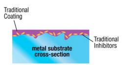
VpCI®-329 D ES attacks corrosion on two fronts. Its oilsoluble corrosion inhibitors first create a tenacious film that clings to metal surfaces, providing excellent contact corrosion protection. VpCIs also release into the air and attach electrochemically to the metal surface. The coating performs effectively even under the adverse conditions of 100% relative humidity and in the presence of such corrosive species as chlorides, hydrogen sulfide, or other sulfur compounds.
