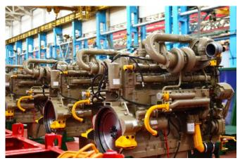
Excellent product performance was also demonstrated when a large engine plant discovered corrosion after they test-ran their new engines for several hours. The water runoff would quickly turn into red rust. They realized this occurred because of poor corrosion prevention in their cooling water system, and they needed to find a more cost-effective
