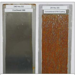
Panels coated at 1.0-1.2 mils DFT and subjected to ASTM B117 Salt Spray Testing
