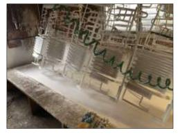
Just last year, Cortec® was able to help a refrigerator coil manufacturer replace a solvent-based coating with a water-based coating for increased worker safety and better corrosion protection. The manufacturer was using the solvent-based paint to coat new refrigerator coils. This exposed workers to a strong solvent smell and associated hazards. To make matters worse, the paint did not
