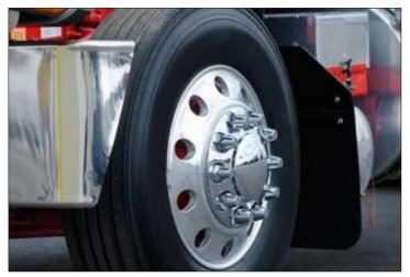
to the end user. The second manufacturer applies VpCI®-391 to numerous corrosion-prone areas—such as keyholes, wheel lug nuts, and points where several different metal parts attach together—on new heavy equipment. The coating provides needed protection while the equipment is shipped or stored outdoors, ensuring it stays in like-new condition without significant changes to vehicle appearance.
