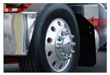
VpCI®-391 has been found to be a useful option especially as a transit coating, allowing users to spray VpCI®-391 as a clear coat right over the top of new firetruck finishes or over corrosion prone components of heavy equipment—lug nuts, dissimilar metal components, keyholes, bolt threads, etc.—without significantly changing the appearance. Testing of VpCI®-391 has found that use of VpCI®-391 on weld joints does not negatively
