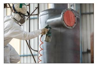
2K products, primers, and multiple coats—in order to achieve the best coating performance possible. That is where <u>VpCI®-395</u> comes in as Cortec's first-class, 2K metal primer for corrosion protection!
