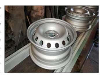
previously rusted, so a coating of CorrVerter® Rust Converter Primer was applied first to passivate the rust, followed by a topcoat of VpCI®-396. The same coatings system was used by a vehicle maintenance company in Croatia that wanted to restore corrosion-damaged wheel rims. This was done by passivating the rust with
