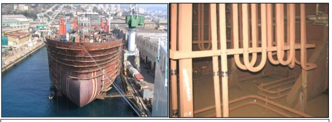
Application of VpCI<sup>®</sup>-645 for hydrostatic testing of 12 ship storage tanks using sea water. It is very important to use products with a lower environmental impact in applications where testing water will be drained into the sea.
