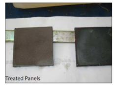
A large producer of boilers and hot wells had numerous corrosion problems during testing, shipping, and storage. Corrosion was slowing down production and they were receiving complaints from customers. VpCI®-645 was used during pressure testing of the equipment. They designed a closed system using water treated with VpCI®-645. After the equipment dried, VpCI®-309 was fogged inside. With this protection the boilers and hot wells were ready for shipping and storage.
