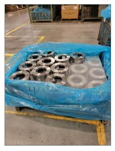
VpCI<sup>®</sup> Film can also expand storage options outdoors when warehouse space is limited. Cortec's outdoor grades of <u>VpCI<sup>®</sup>-126 HP UV Shrink Film</u> and <u>MilCorr<sup>®</sup> VpCI<sup>®</sup> Shrink Film</u> can create perfectly acceptable individual outdoor storage units that offer much better corrosion protection than basic tarps.
