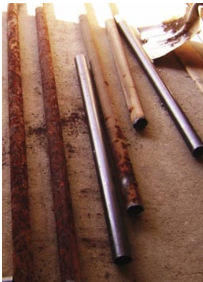
New boiler tubes (shiny) alongside old tubes damaged from corrosion that could be the result of a non-existent or inadequate preservation program. Cortec® image.
