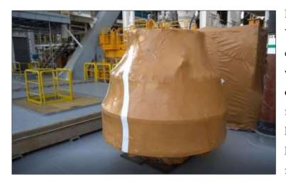
In addition to corrosion protection, MilCorr® VpCI® Shrink Film is UV resistant and has an excellent track record for withstanding severe weather like hurricanes. When used on an offshore platform that took an almost direct hit from Hurricane Harvey in 2017 in the Gulf of Mexico, none of the MilCorr® VpCI® Shrink Film came off, and the equipment was still found to be protected and corrosion-free at the
