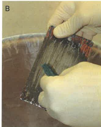
Fig. 4 — A — Organic acid rust remover gel clinging to a vertical surface; B — using a scrub pad to remove rust after a second application.
