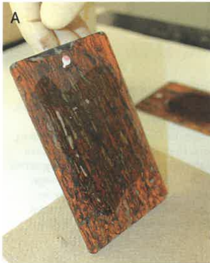
Fig. 4 — A — Organic acid rust remover gel clinging to a vertical surface; B — using a scrub pad to remove rust after a second application.
