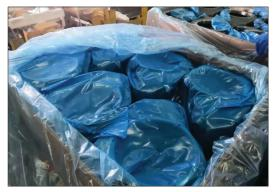
VpCI® Bags are a great way to protect metals from corrosion. They can hold everything from large engines to small nuts, bolts, and instrument strings. While VpCI®-126 Shrink Film is a great option for shrink wrapping and storing large items, premade bags are even more convenient for packaging and corrosion protection. These bags come in many sizes-small to largeand different styles. The choice remains up to you — which bag do you want? Here's a look at some of the options:
