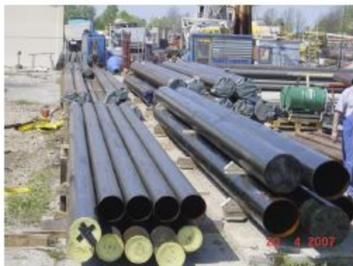
Figure 1. The internal and external surfaces of the pipes were washed with VpCI™-414. The inside surfaces were sprayed with VpCI-369D and the external surfaces were coated with VpCI-368M. Both ends of the pipes were sealed with a plastic cap or film.
