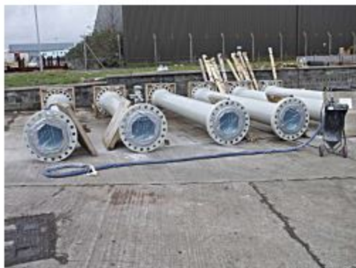
Figure 2. After the application of Cortec® products, the pipes are stored for three years.
