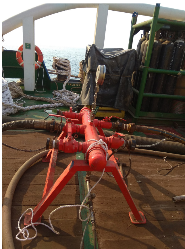
Figure 6. Using a pressure gauge to monitor VCI application. Image courtesy of Cortec Middle East.
