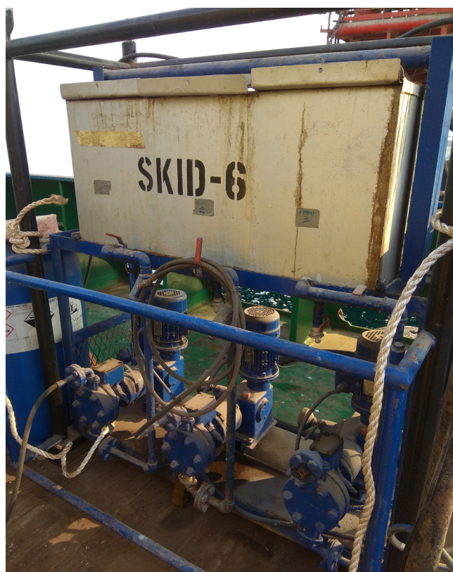
Figure 5. VCI fogging fluid was injected into the skid using nitrogen pressure. Image courtesy of Cortec Middle East.
