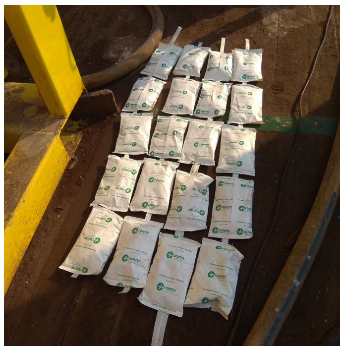
Figure 3. Breathable pouches containing VCI. Image courtesy of Cortec Middle East.
