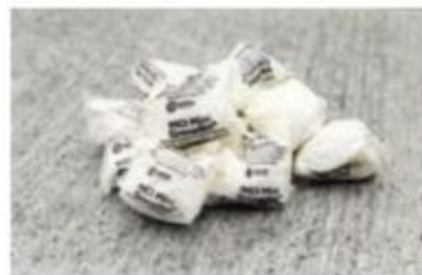
Designed to protect steel and other metals used in the construction industry, Cortec's MCI Grenades consist of migrating corrosion inhibitors (MCIs) packaged in EcoSol water-soluble PVA bags, which quickly dissolve upon contact with water in the concrete mix.
