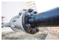
transit applications where pipes and flanges may be repeatedly handled. For the most extreme conditions, VpCI-368 offers even heavier-duty protection. This fast-drying solvent-based coating leaves a slightly brown waxy finish and should be removed prior to flange installation using an alkaline cleaner from the VpCI-41x Series.
