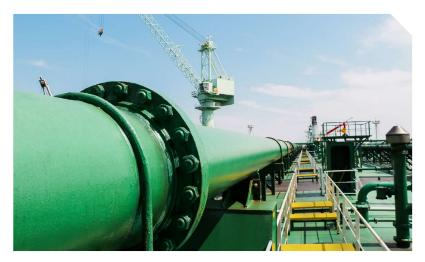
ipes for the marine environment are built specially, with several types of pipes used. They are used in different mechanical operations on ships as well as in offshore systems. Harsh atmospheric conditions in marine environments expose pipes to high corrosion levels. Removable coatings are an excellent way to ensure faster installation and less downtime by keeping corrosion at bay.
