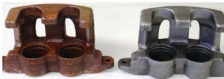
Non-toxic rust removers such as VpCI-422 can effectively clean the rust off parts to restore them to usable condition on the same day.
