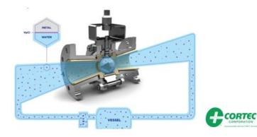
VpCI<sup>®</sup> s have a unique advantage over traditional corrosion inhibitors and rust preventatives because they do not need to be applied directly to the surfaces they protect. They are able to vaporize from a source material, disperse throughout an enclosed space, and condense on metal surfaces, even in intricate, hard-to-reach areas.
