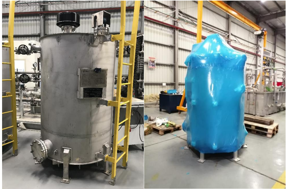
After parts were padded with VpCI 132 Foam, Cortec's VpCI®-126 HP UV Shrink Film was wrapped and heat shrunk around the equipment.
