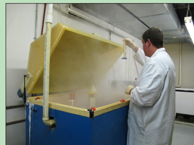
Eric Uutala, Tech. Service Engineer, analyzing a product in the humidity chamber.
