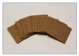
In addition to wrapping metal parts for protection, VpCI® paper can be used for lining crates or interleaving metal parts in larger containers. They can also be inserted inside metal void spaces to protect component internals. For example, VpCI®-143 Paper Emitters are 1" x 1" (6.45 cm²) squares coated on two sides with VpCI® coating. They protect up to 25 cubic inches (410 cm³) of space and are easy to slip inside a small package or metal
