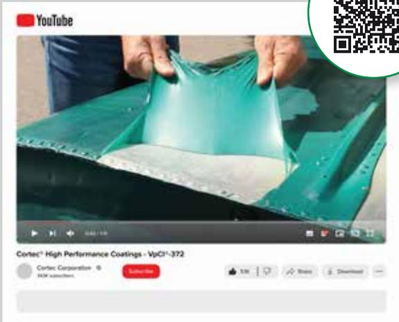
Cortec® offers innovative removable coatings that look and perform like paint but can be easily removed when needed. These coatings are ideal for transit and temporary storage, especially for complex-shaped items.
