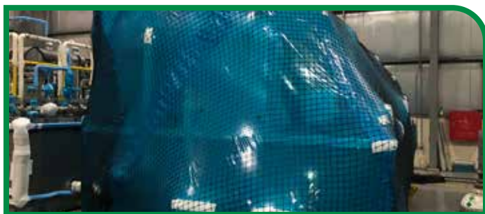
PRESERVATION OF LUBE OIL SKIDS Case History #772
