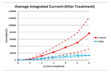
Results of the US Bureau of Reclamation M-82 (M0820000.714) Standard Protocol to Evaluate the Performance of Corrosion Mitigation Techniques in Concrete Repairs. Results are of MCI®-2020 applied under a standard sealer.
