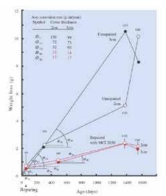
control samples. Applying MCI®-2020 after cracks appeared worked very well to reduce corrosion rates in samples.
