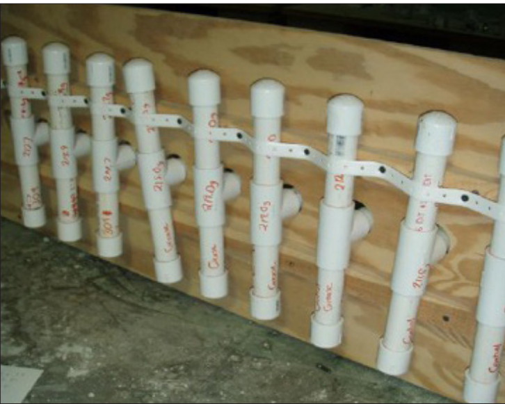
Figure 3: Corrosion Test Setup, Pennsylvania State University Grouting Laboratory Report
