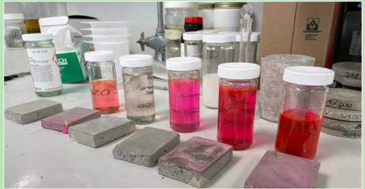
Concrete samples treated with MCI® SACI and fugitive die before QUV testing.
