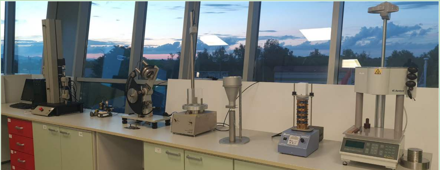
Left to right at EcoCortec®: Oakland Instrument MT-1528 for Tensile Strength/Elongation, Elmendorf Tearing Tester, Oakland Instrument for Dart Drop Impact (new), SCITEQ bulk density tester, Gilson Company Performer III 3" Sieve Shaker SS-3 (new), Dynisco D 4002 Melt Flow Indexers.
