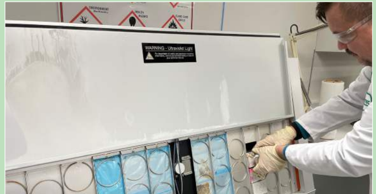
Colin placing the concrete samples with fugitive die facing inward to where they will be exposed to accelerated weather testing.
