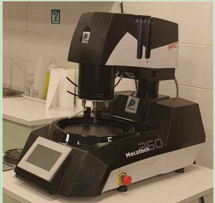
Plug polisher for VIA testing according to NACE TM-0208 or Cortec® method.
